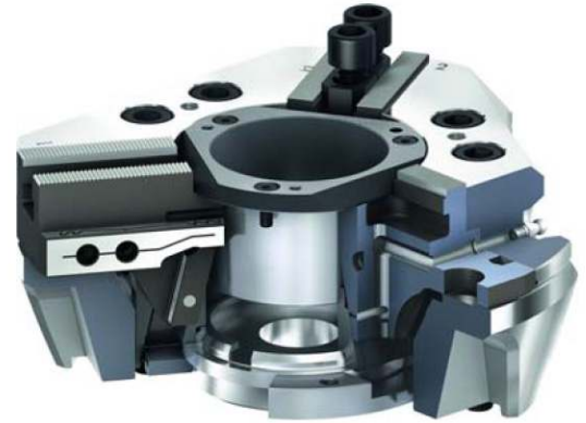
Figure 6: The axially displaceable piston transmits the force to the base jaws and generates a radial jaw movement synchronous to the axis of rotation.
