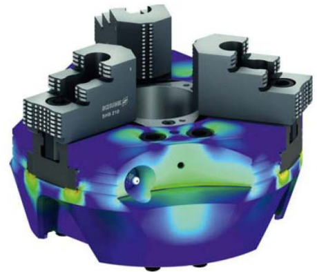
Figure 4: FE parameter optimization for reduced notch stresses and highest stiffness.
