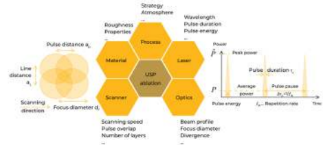
Figure 1. The ultra-short pulse ablation is influenced by a multitude of parameters.
